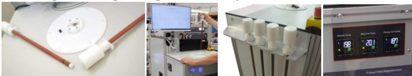
Above: PFM08-10 AT sample holder stick, a PFM08-10 AT in operation. Samples stick storage on the side of the PFM08-10 and sample temperature measurement displays.
