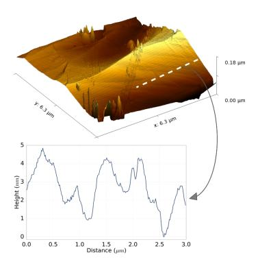
3D topography showing phase transformation-induced changes of topography up to 5 nm as shown by the line cross section in transformed areas.
