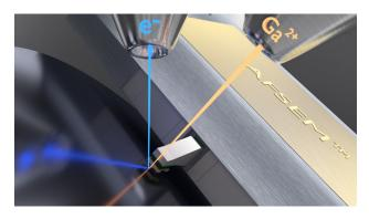
Schematics of correlative analysis in a dual beam system using SEM, FIB, and AFSEM® in an interactive experiment.
