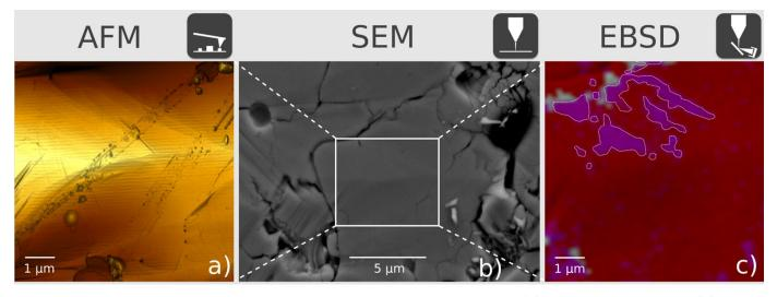
AFSEM™ enables correlative EBSD and AFM topography analysis. AFM image (a), correlative SEM image (b) and EBSD crystallographic analysis of ZrO<sub>2</sub> sample (c). Sample courtesy: Prof. Y. Zeng (SICCAS, China)
